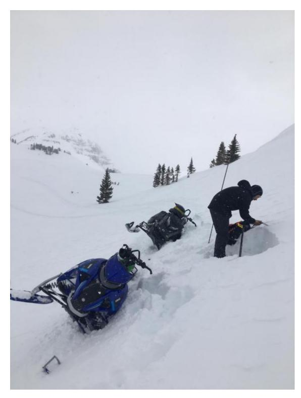
Ian and Dave stop to do a quick stability test as they hunt for a layer of weak snow 1-2 feet under the surface. Photo: GNFAC
