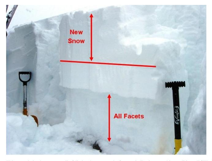
This extended column test easily failed and propagated a fracture indicating unstable conditions (ECTP 15). Weak faceted crystals have been heavily stressed by new snow that has nearly doubled the snowpack depth. Many slopes have a similar snowpack.
