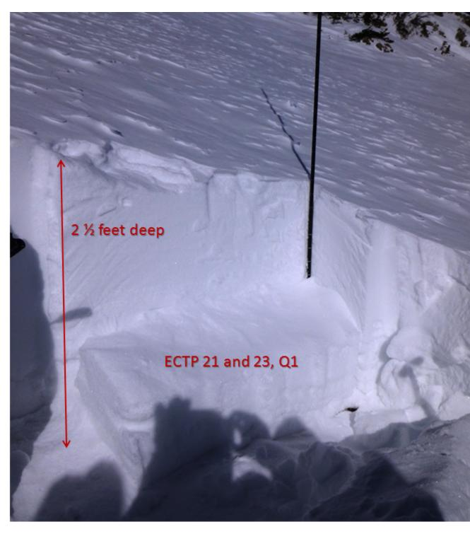
This pit was dug on a 32 degree southeast facing slope. Facets 33cm off the ground (total depth 85cm) broke clean in stability tests (ECTP 21, 23, Q1). Thin snowpacks are holding weaker snow that avalanched on a couple slopes in the northern Bridgers on Thur and Fri. Photo: GNFAC
